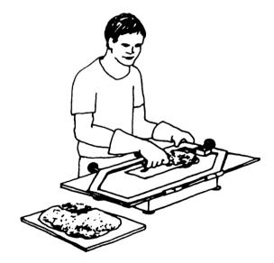
Figure 2: Work the mortar mix under vibration
