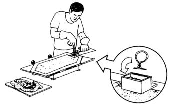
Figure 4: Fill nib forming box and insert loop of wire
